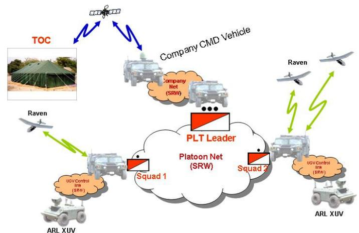
TC software resided at the Squad vehicle at Ft.Dix. Group commander software resided at the TOC (communicating over a SATCOM or SRW link) or Company command vehicle.
